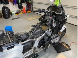
The OEM filter wasn't even that dirty! It had some grit and dust on it but was in no way impeding performance, Anyway I installed a new K&N air filter and started reassembly the next day. That involved another 6, frustrating and tiring hours. Honda could have done a better job of placing that air filter since they recommend replacing it at 16k intervals (like that's going to happen)! I hate to think of what the bike shop would charge to do the job!
